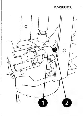
STARTING MOTOR DISASSEMBLY Disassembling drive-end bearing Prise cap (1) off commutator end shield. Mark installation position of drive-end bearing and commutator end shield with respect to stator frame. Slacken off bolts (2).
